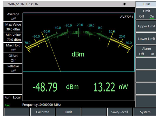
Power Measurement (USB Power Sensor)
